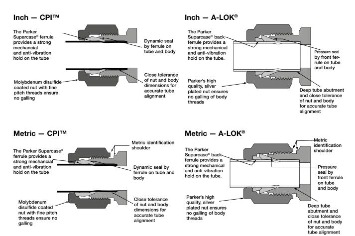
Parker Instrumentation Tube Fittings are supplied complete and ready to use. The ferrule(s) swage onto the tube as it moves down the body seat creating a pressure/vacuum-tight seal on both tube and body by the interface pressure and surface finish of mating components. The Parker Suparcase™ ferrule (backferrule only on A-LOK®) creates a strong mechanical hold on the tube.
